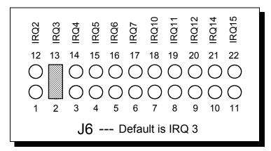
Figure 6 --- Interrupt level (IRQ) selection
